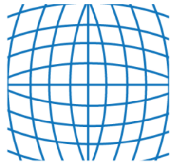
positive radial distortion "barrel"
